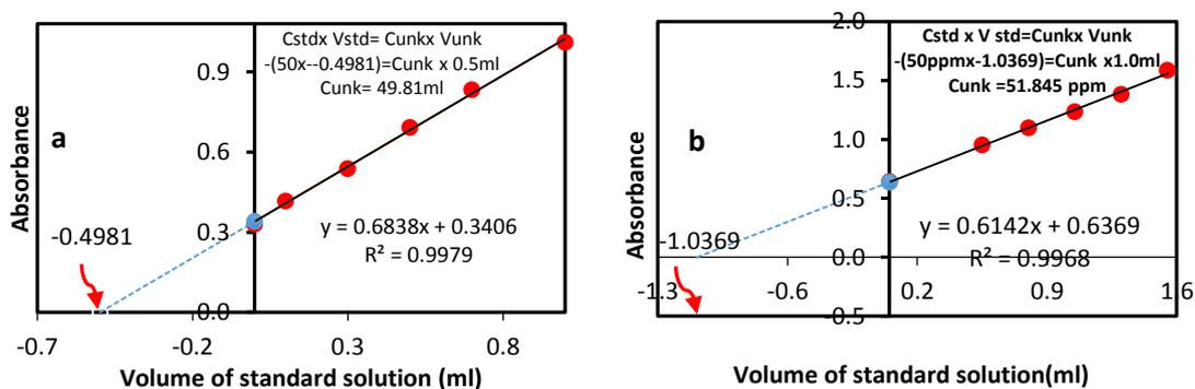
Figure (9): Determination of CLNZ in tablet (Rivotril) by SAM
