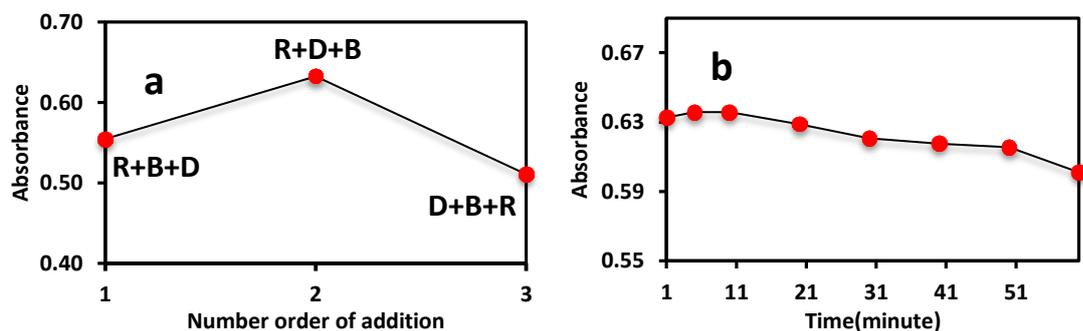
Figure (5): (a) Effect of order of addition (D: Drug, R: Reagent, B: Base) (b) Effect of time on the stability of CLNZ- *p*-Br complex ( $10\mu\text{g}\cdot\text{mL}^{-1}$ ).
