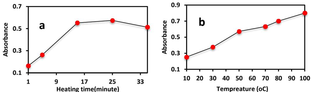
Figure (4): (a) Effect of heating time. (b) Effect of temperature on the absorbance of  $10\mu\text{g}\cdot\text{mL}^{-1}$  of CLNZ.
