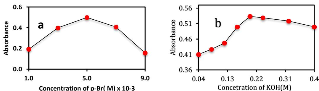
Figure (3): (a) Effect of *p*-Br concentration. (b) Effect of KOH concentration on the absorbance of  $10 \mu\text{g.mL}^{-1}$  of CLNZ.
