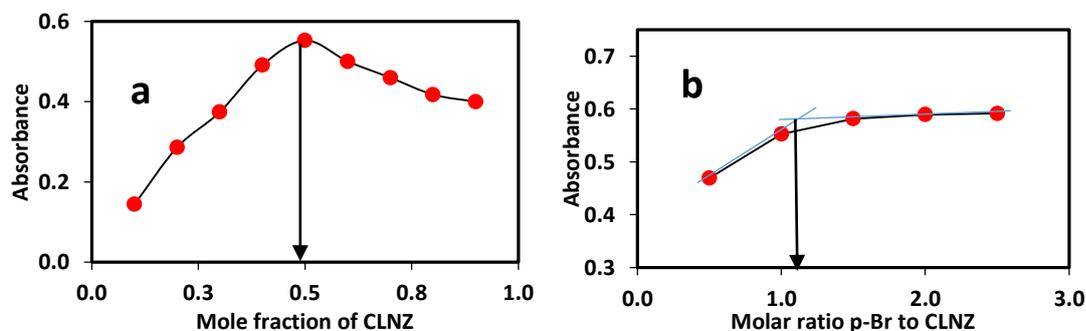
Figure (7): (a) Job's method of continuous variation (b) Mole ratio method ( $[\text{CLZ}], [p\text{-Br}] = 1.5 \times 10^{-5}\text{M}$ ,  $\lambda_{\text{max}} = 387\text{nm}$ ).
