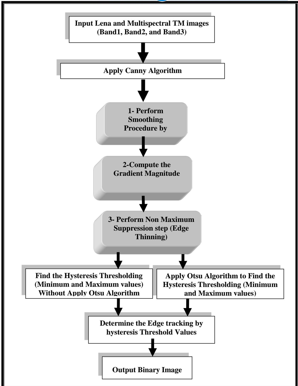
Figure No. (2) Block Diagram Summarizes the Procedure Steps for the Adaptive Canny Technique
