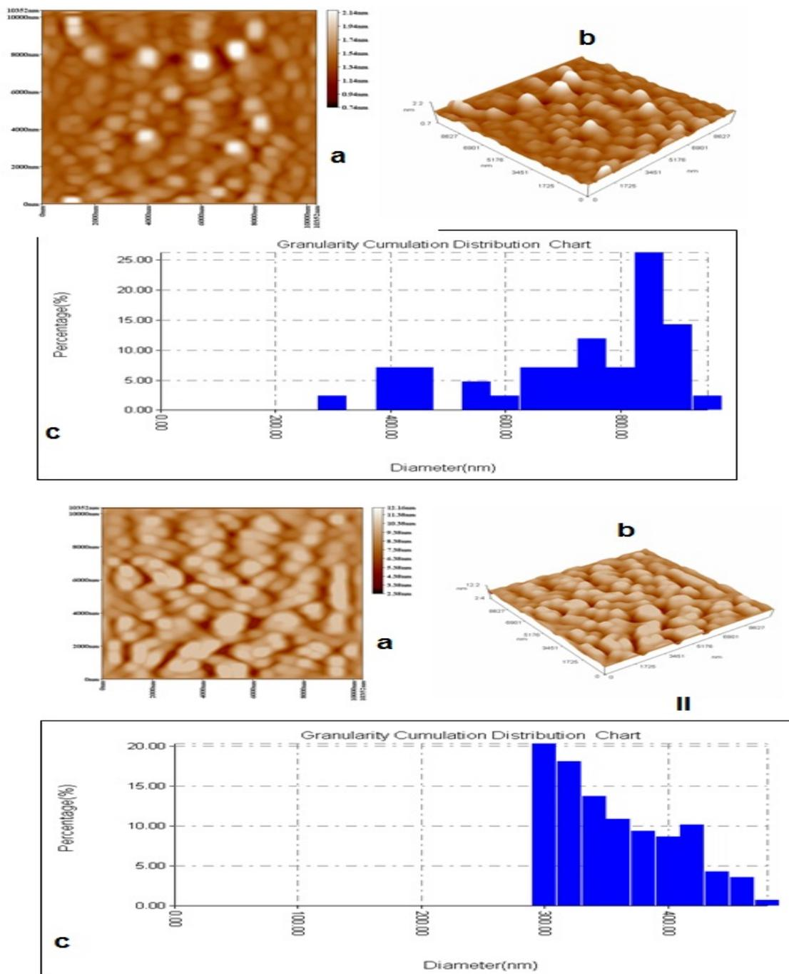
**Fig. (2):(I) AFM images of clay. (II) AFM images of Fe-BNC clay (a)The 2D, cross section (b) 3D and (c) Pore size distribution diagram**
