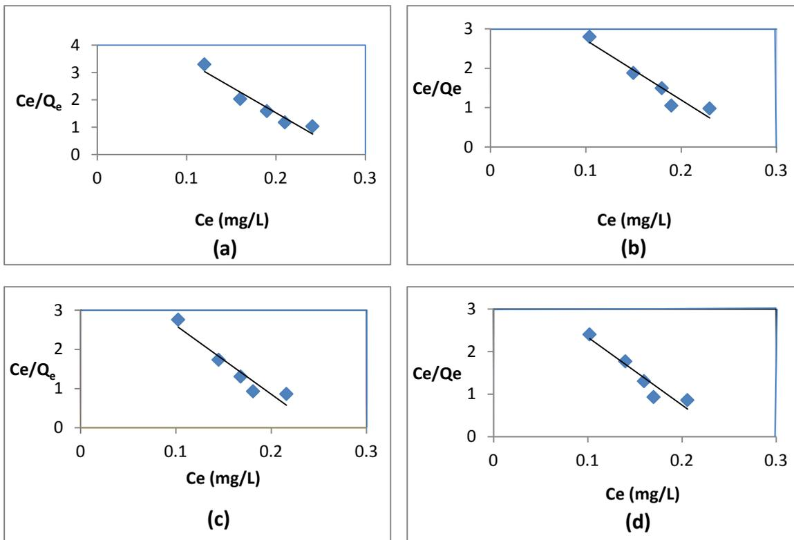
Fig. (7): Langmuir's isotherm plot for the adsorption of BG on Fe-BNC [(a) 283, (b) 293, (c) 298, (d) 303K]
