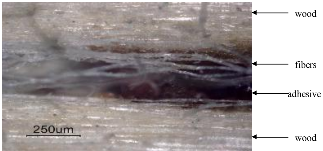
Fig.(2): The optical micrograph(100x) of wood- adhesive - wood reinforced with mat fibers
