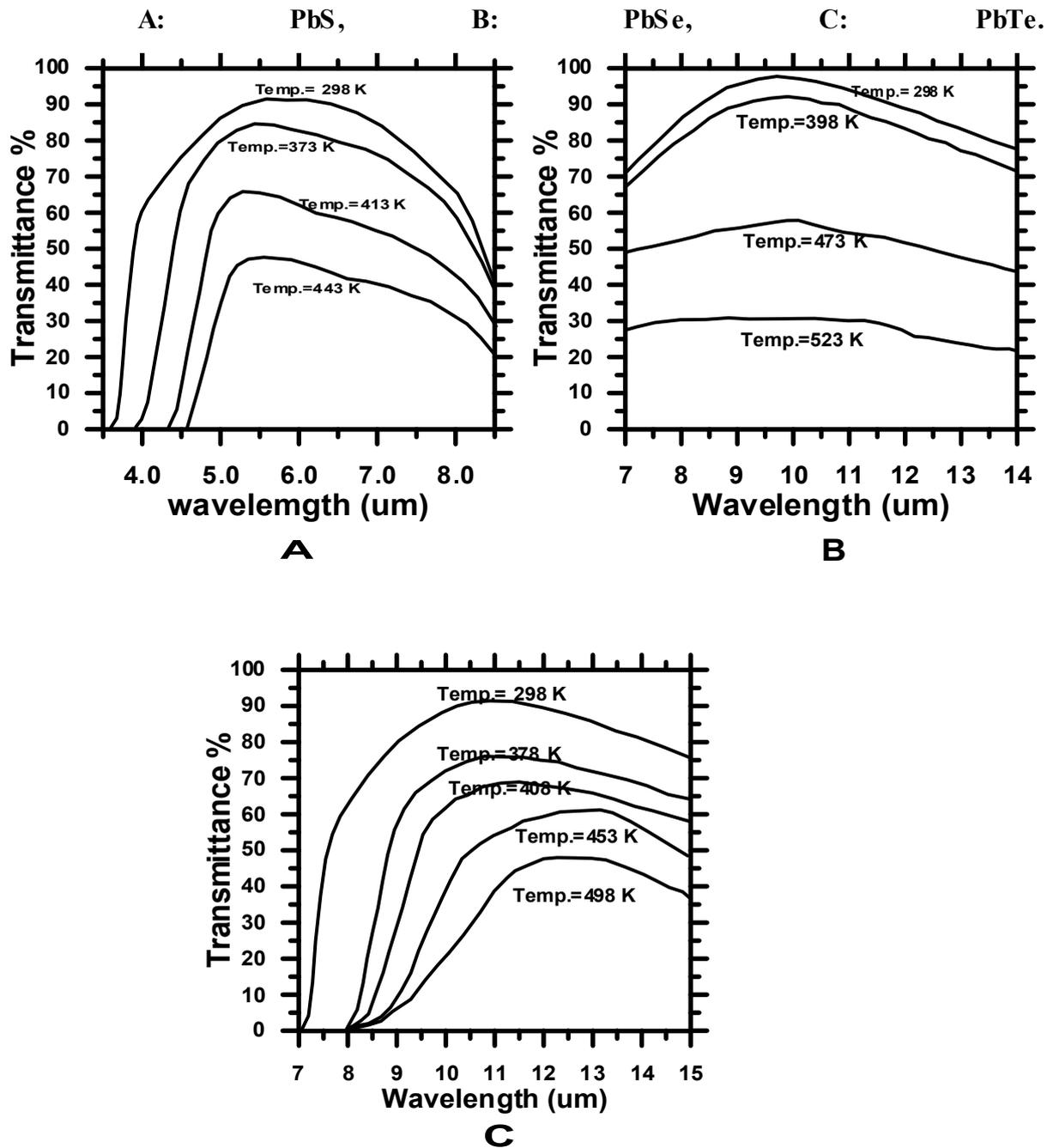
**Fig.(1):** Experimental transmittance versus wavelength for different temperatures.
