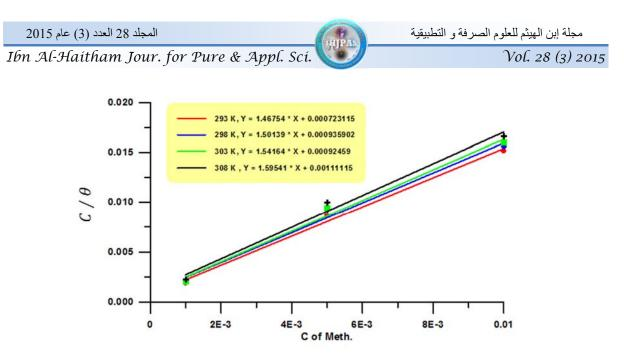
Fig. (4): Langmuir adsorption plots of L-methionine on the pure Al in 0.6 mol.dm<sup>-3</sup> NaCl solution at various temperature.
