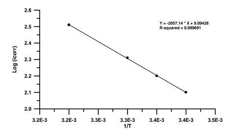
Fig. (2): Arrhenius Plot relating Log (i<sub>corr</sub>) to 1/T for the corrosion of pure Al in the pH = 0.7 in presence of (0.6 mol.dm<sup>-3</sup>) NaCl over the temperature range (293 – 308) K.
