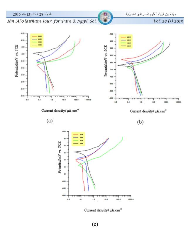
Fig. (3): The typical polarization curves of pure Al in with (0.6 mol.dm<sup>-3</sup>) NaCl solution containing of L-methionine as inhibitor (a= 1×10<sup>-3</sup>, b = 5×10<sup>-3</sup>, c =1×10<sup>-2</sup> mol.dm<sup>-3</sup>) over the temperature rang (293-308)K.
