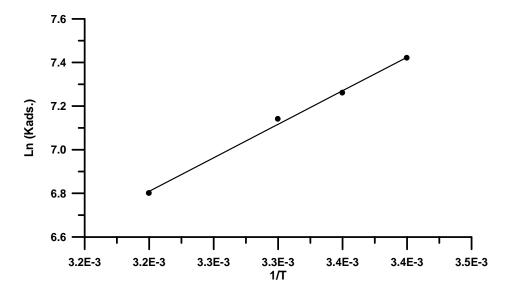
Fig. (5):Van't Hoff plot pure Al in 0.6 mol. dm<sup>-3</sup> NaCl solution containing L-methionine in pH = 0.7
