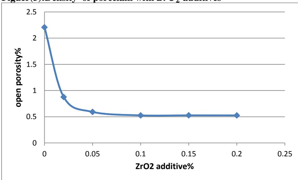
Figuer(6):porosity of porcelain with  $ZrO_2$  additives
