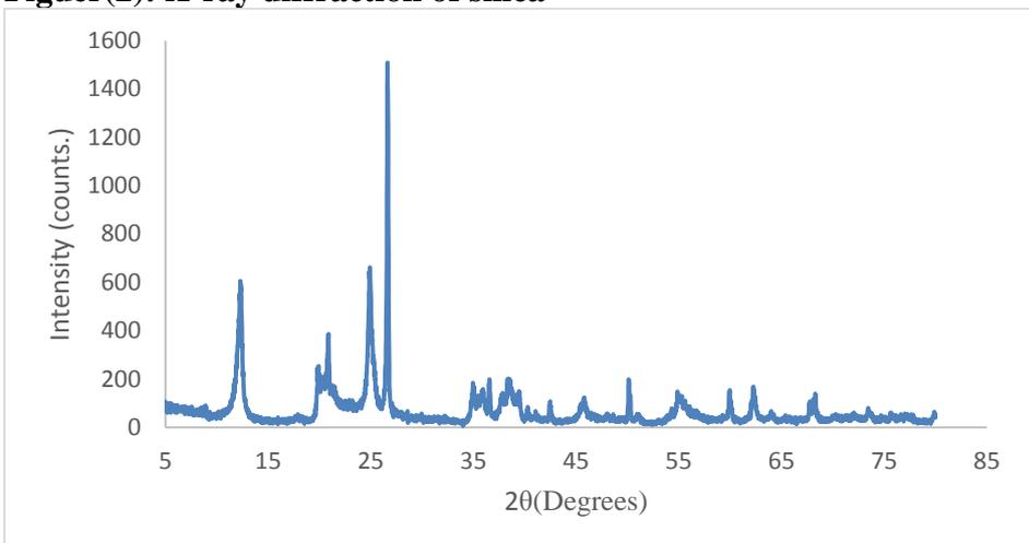
**Figueru(3): X-ray diffraction of kaolin**
