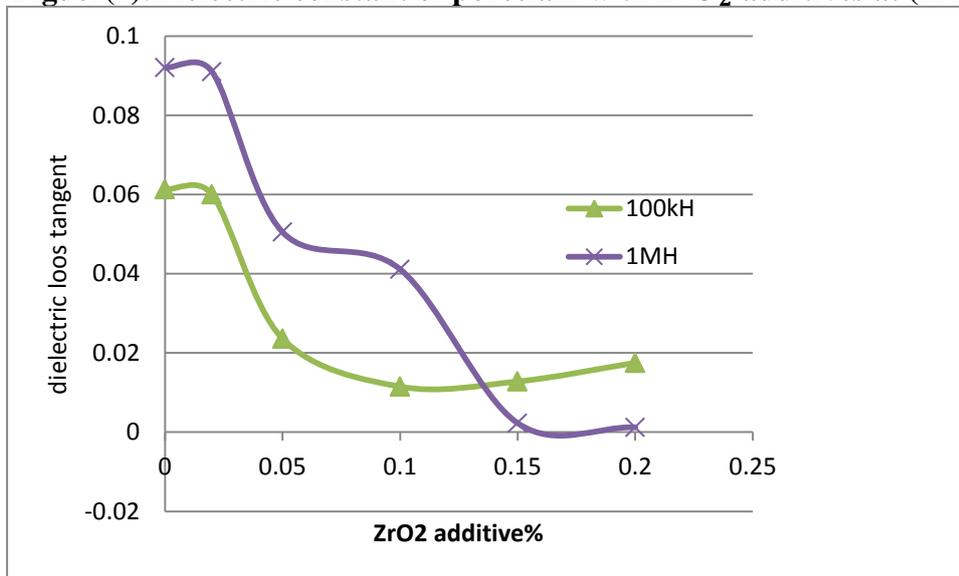
Figure(8):Dielectric loss tangent of porcelain with  $ZrO_2$  additives at (1MHz) and (100KHz)
