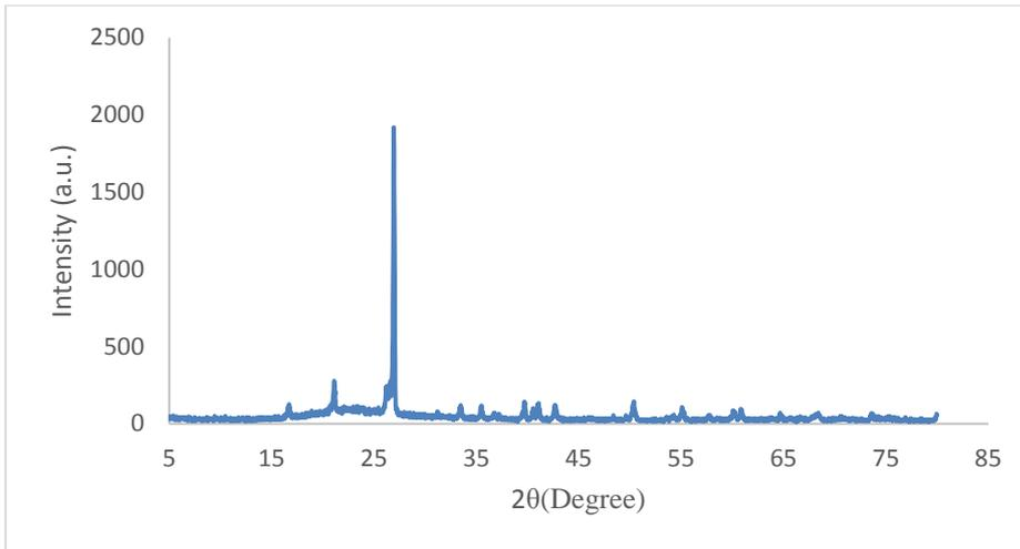
Figuer(4): X-ray diffraction of composition (kaolin , feldspar, silica)
