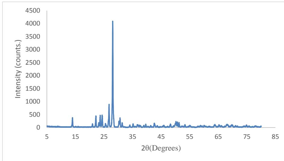
**Figuer(1): X-ray diffraction of Feldspar**
