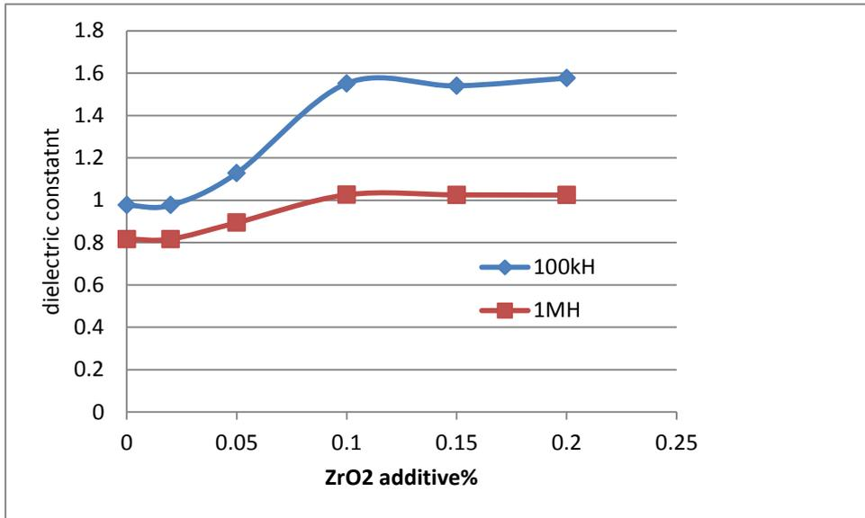
Figure(7):Dielectric constant of porcelain with  $ZrO_2$  additives at (1MHz) and (100KHz)
