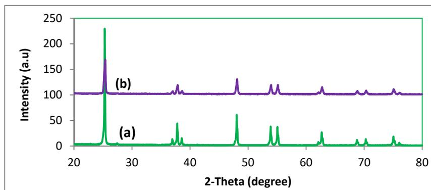
Figure (8): XRD of (a) pure TiO<sub>2</sub> and (b) TiO<sub>2</sub>- *S. reginae*
