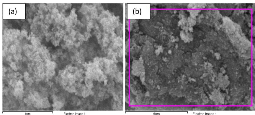
Figure (6): SEM images of (a) pure TiO<sub>2</sub> and (b) TiO<sub>2</sub>- *S. reginae*
