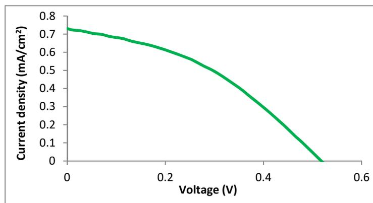
**Figure (9): Photocurrent–voltage curve for DSSC sensitized with *S. reginae* extract**
