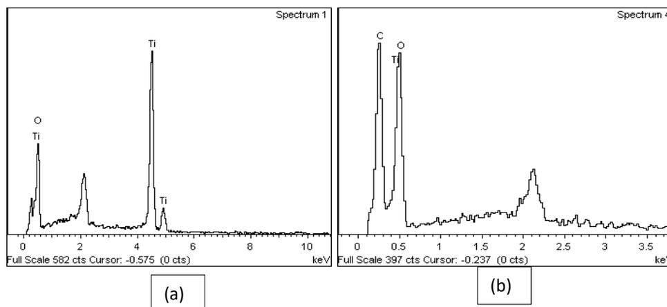
**Figure (7): EDX spectra of (a) pure TiO<sub>2</sub> and (b) TiO<sub>2</sub>-*S. reginae***
