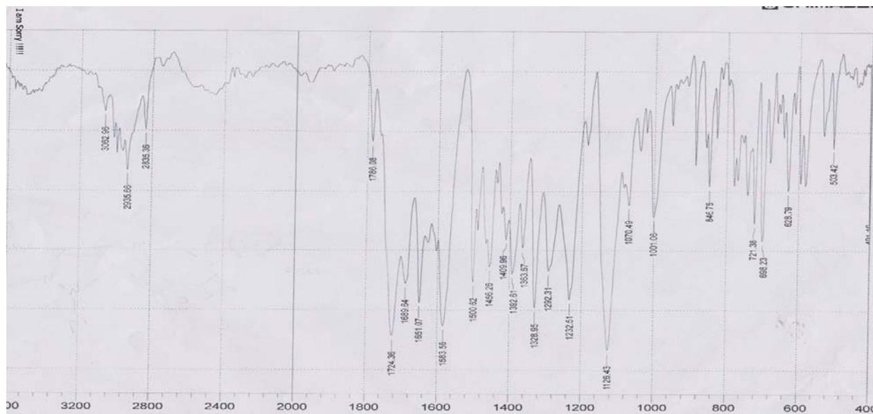
**Figure (8): IR spectrum of Schiff base compound ( 9)**
