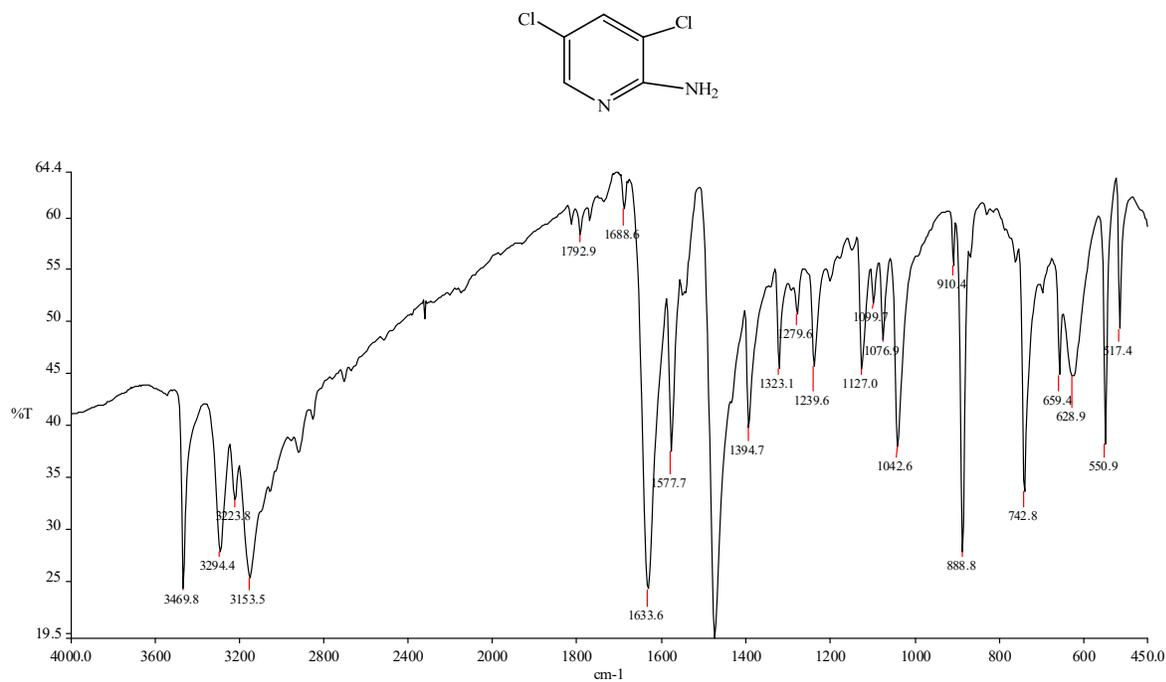
Figure(1): IR spectrum of 2-amino 3,5- dichloropyridine
