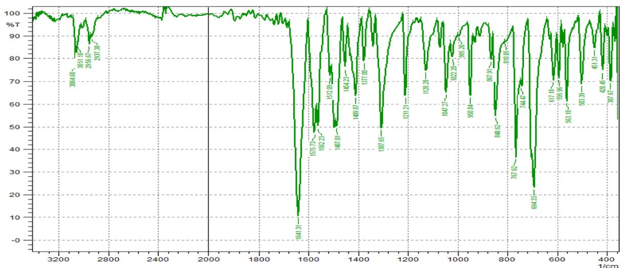
**Figure (5): IR spectrum of Schiff base compound (8).**
