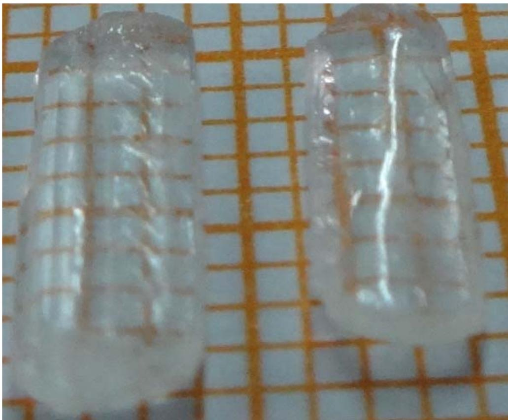
**Figure No. (1a): pure crystal of  $K_2SO_4$**
