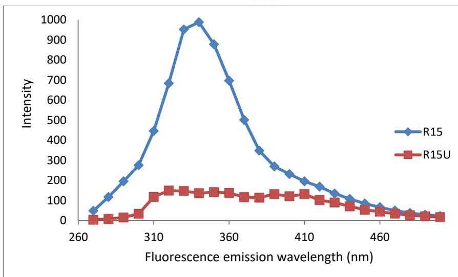
**Figure (4): Comparing the fluorescence spectra for 1.295 mg/l of R15 vs. R15u oil samples in hexane**
