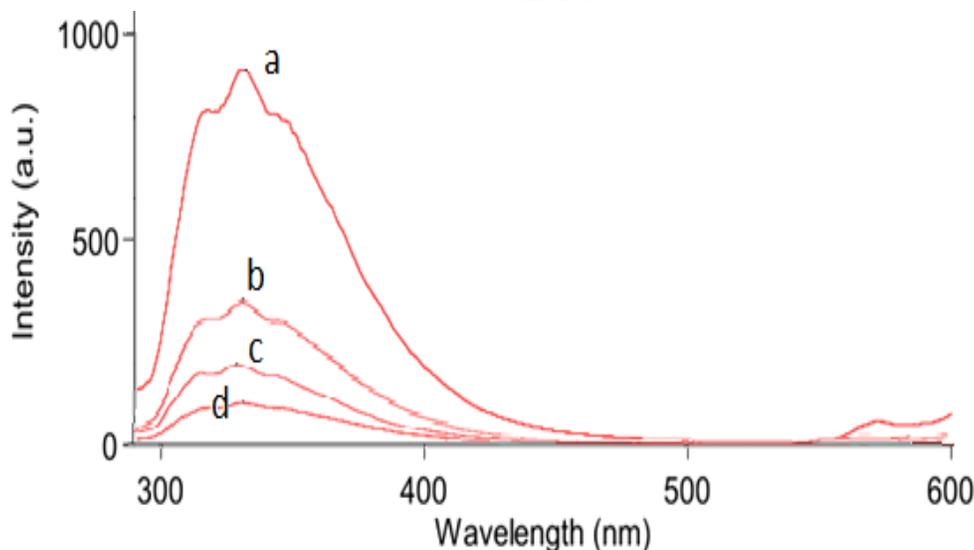
**Figure (6):** Overlay fluorescence spectra for the following slits widths a: (ex10, em5), b: (ex5, em5), c: (ex10, em2.5), d: (ex2.5, em5) in nm. Oils were dissolved in ethanol.
