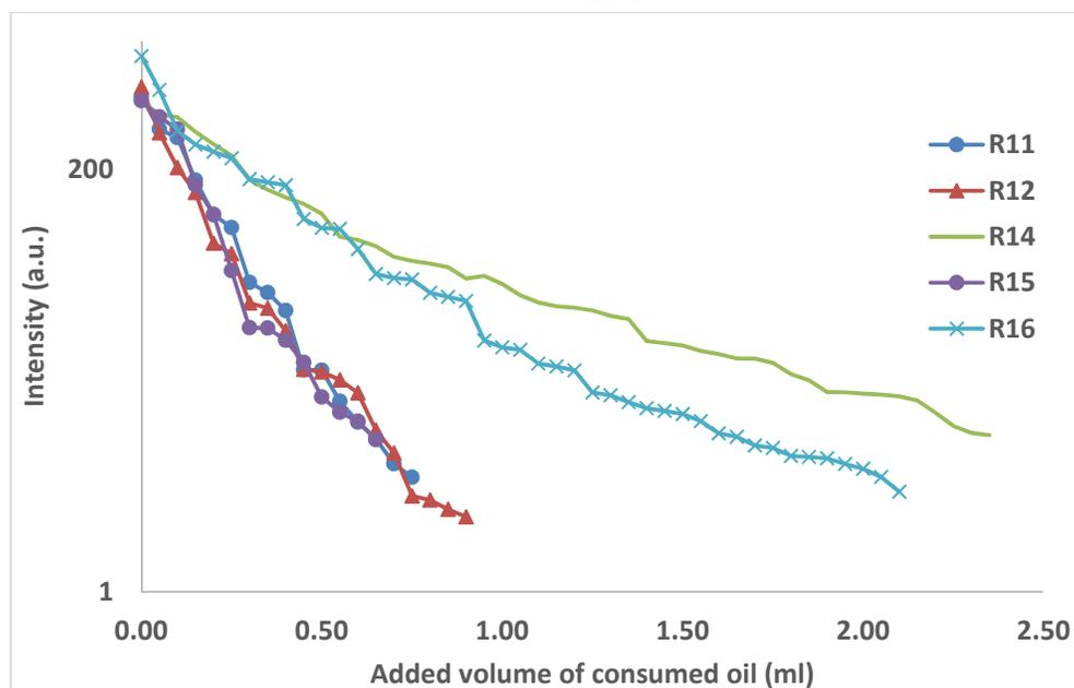
**Figure (23): A comparison for the logarithmic scale to the base 10 of fluorescence intensity of some fresh oils (1.5 ml each) versus an added volume of its peer consumed oil**
