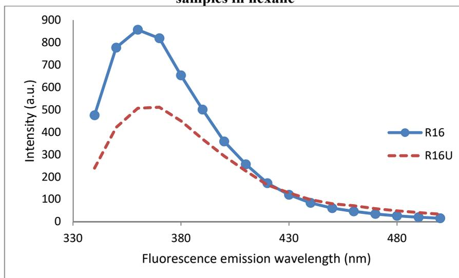
**Figure (5): Comparing the fluorescence spectra for 2.59 mg/l of R16 vs. R16u oil samples in hexane**
