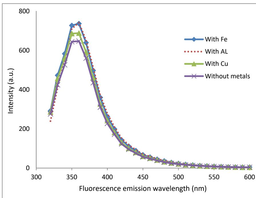
**Figure (20):** Fluorescence spectra for 1.295 mg/l of R16u in hexane with traces of different metals
