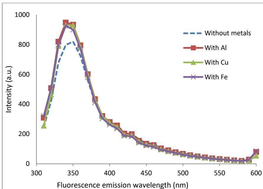
Figure (18): Fluorescence spectrum for 2.59 mg/l of R15u in hexane with traces of different metals
