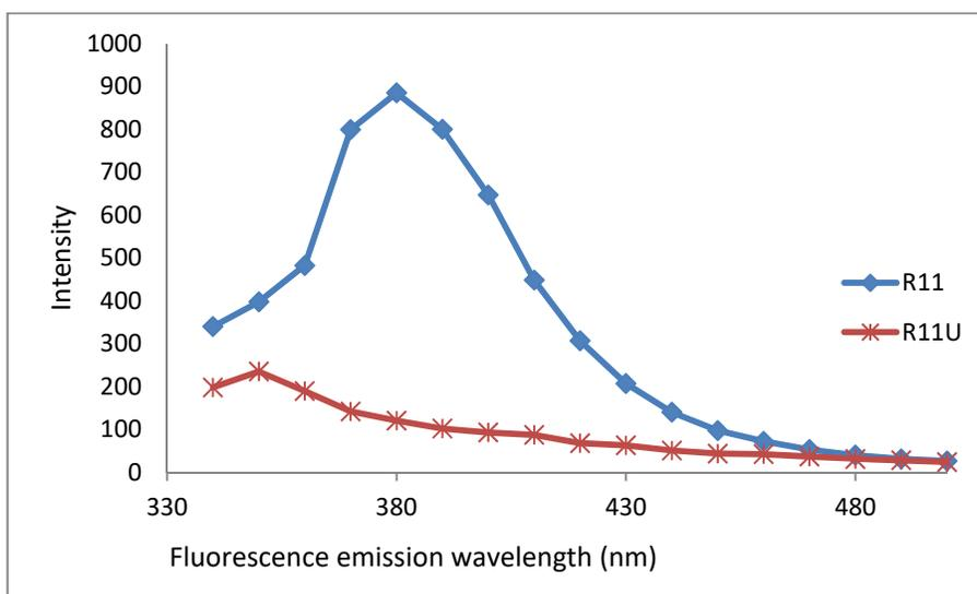
Figure (1): Comparing the fluorescence spectra for 5.18 mg/l of R11 vs. R11u oil samples in benzene
