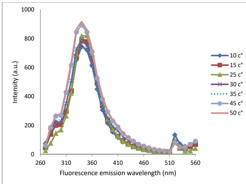
Figure (13): Fluorescence spectra for 1.295 mg/l of R15 in hexane at different temperatures. The best intensity obtained at 50C°
