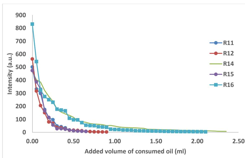
**Figure (22): A comparison for the fluorescence intensity of some fresh oils (1.5 ml each) versus an added volume of its peer consumed oil**
