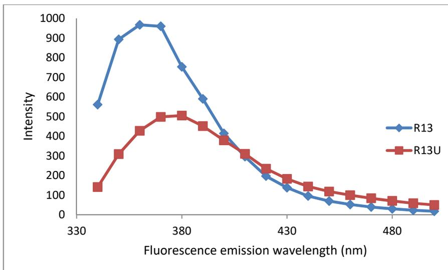
**Figure (2):** Comparing the fluorescence spectra for 2.59 mg/l of R13 vs. R13u oil samples in toluene
