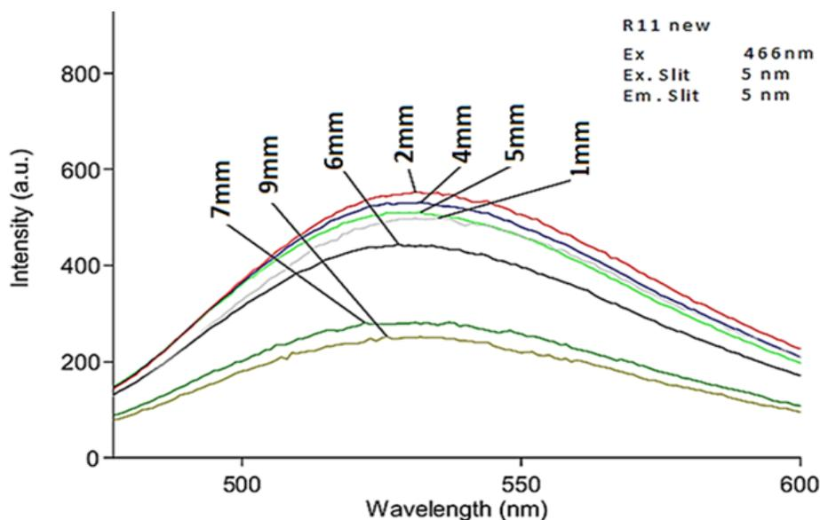
Figure (10): Fluorescence intensity versus emission path length
