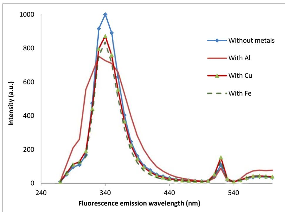
Figure (17): Fluorescence spectra for 1.295 mg/l of R15 in hexane with traces of different metals
