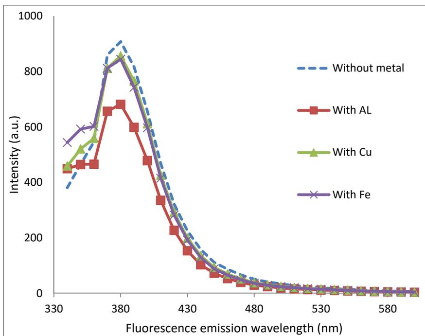
Figure (15): Fluorescence spectra for 5.18 mg/l of R11 in benzene with traces of different metals
