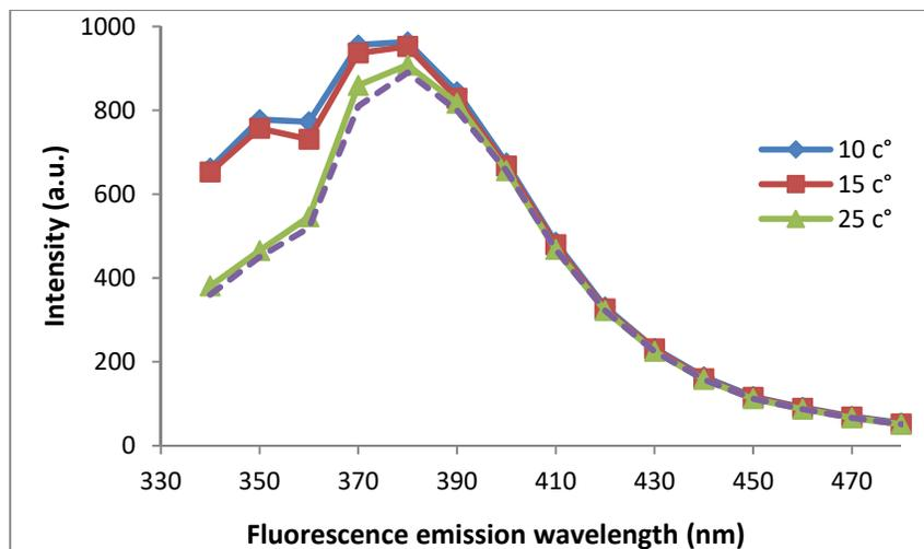
Figure (11): Fluorescence spectra for 5.18 mg/l of R11 in benzene at different temperatures, best intensity obtained at 10 °C
