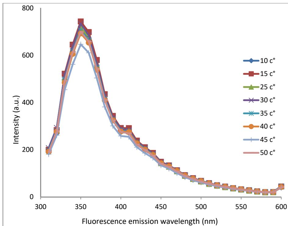
Figure (12): Fluorescence spectra for 1.295 mg/l of R11u in toluene at different temperatures, best intensity obtained at 15°C°
