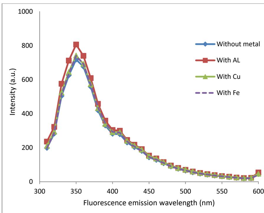
Figure (16): Fluorescence spectra for 1.295 mg/l of R11u in toluene with traces of different metals
