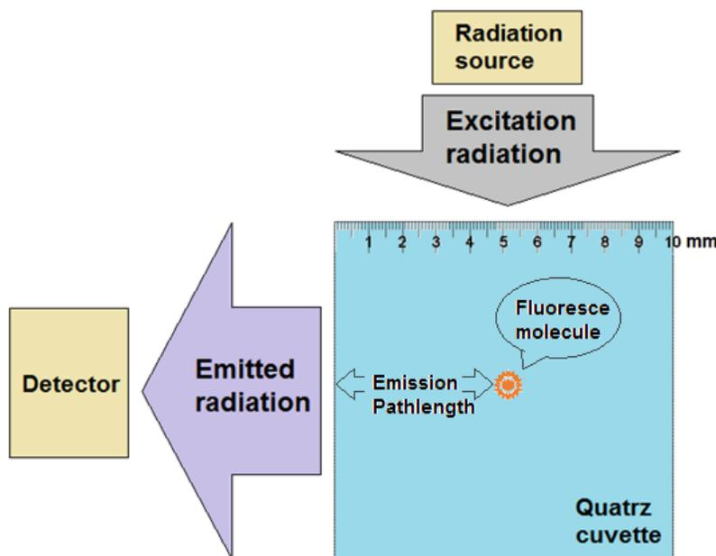
**Figure (8): Controlling the emission path length by shifting the cuvette**
