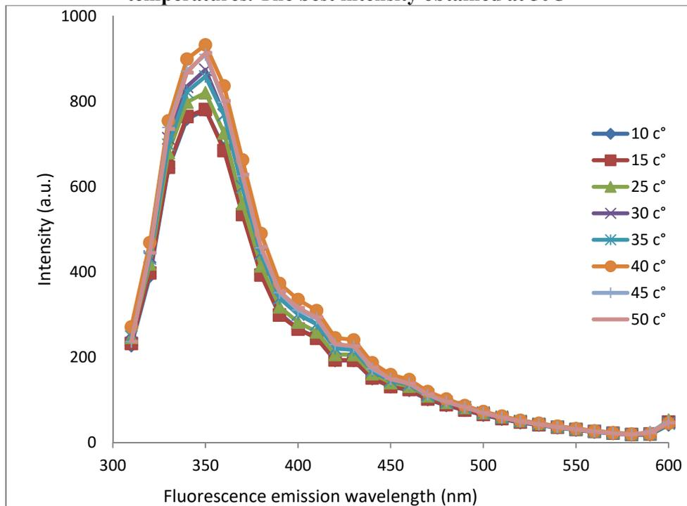
Figure (14): Fluorescence spectra for 2.59 mg/l of R15u in hexane at different temperatures. The best intensity obtained at 40C°
