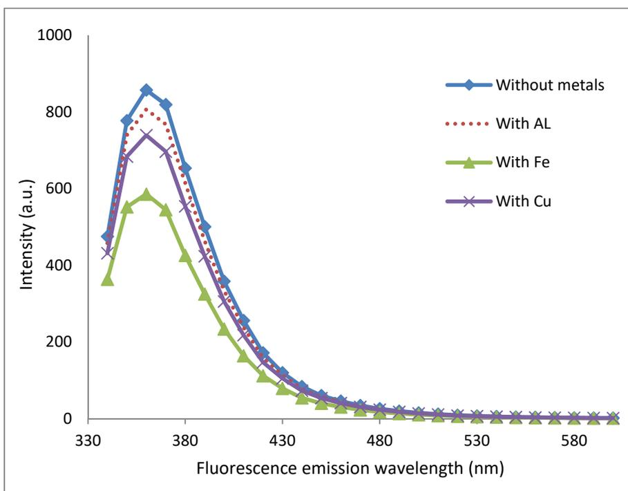
Figure (19): Fluorescence spectra for 2.59 mg/l of R16 in hexane with traces of different metals
