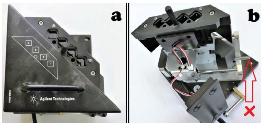
**Figure (7):** Varian Peltier Multicell 4 Position Cell Holder from Agilent Technology; a) a top view, b) partially dissembled, x) manual fine adjustment knob
