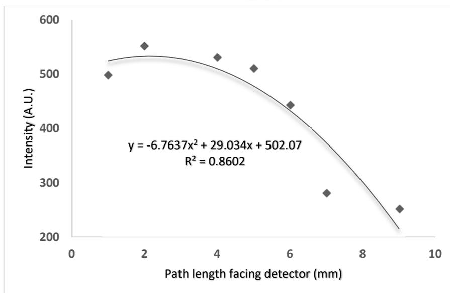
Figure (9): Fluorescence intensity of the oil samples is inversely proportional to the emission path length facing the detector
