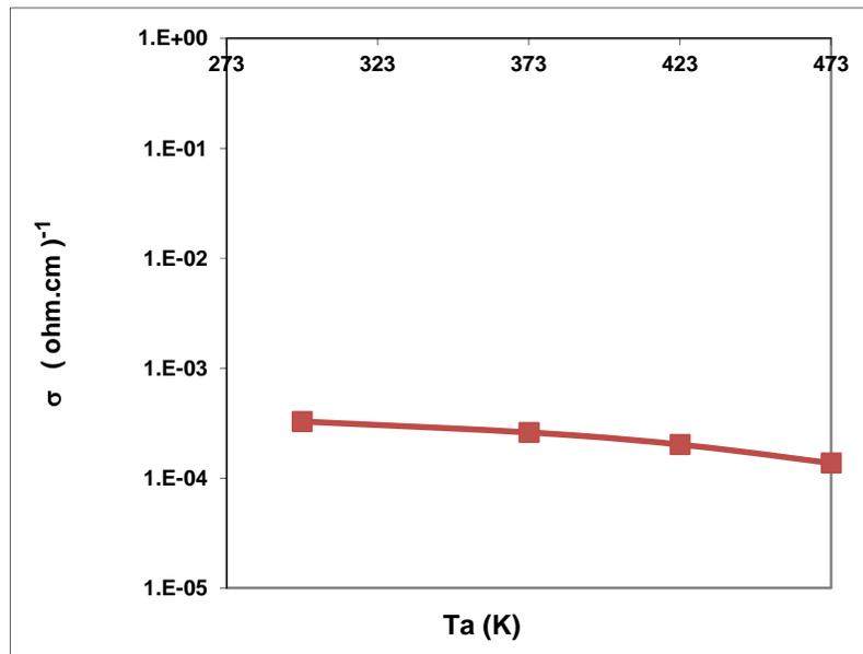
Figure No.(5): Electrical conductivity as a function of annealing temperature for (CdTe) films
