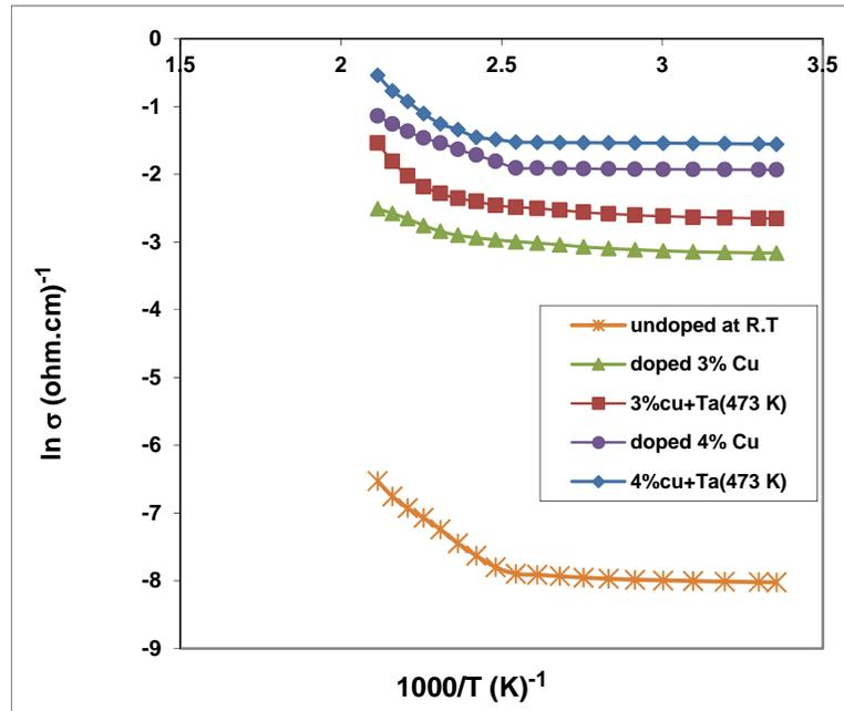
Figure No. (7):  $\ln \sigma$  versus  $10^3/T$  for (CdTe) films un-doped and Cu-doped before and after annealing.
