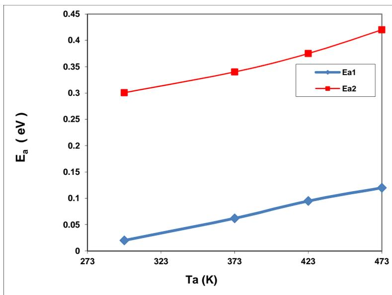
Figure No.(6): Activation energies as a function of annealing temperature for (CdTe) films
