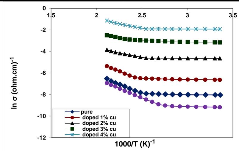
**Figure No.(1): Variation  $\ln\sigma$  versus  $10^3/T$  as a function of doping ratio for (CdTe) films**
