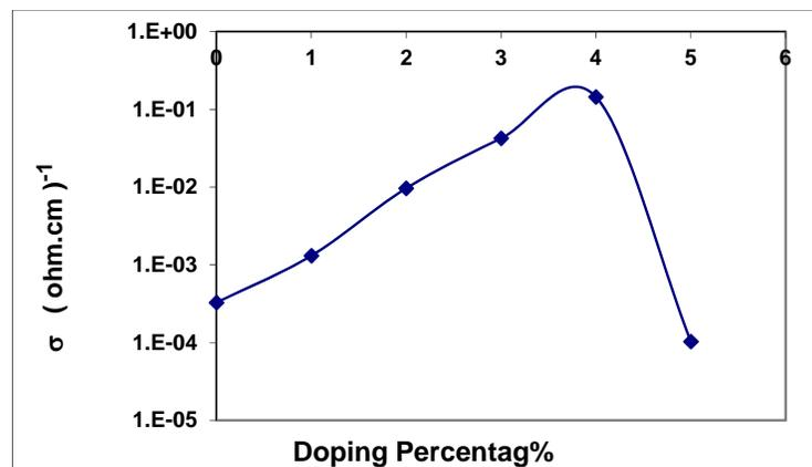
**Figure No.( 2): Electrical conductivity as a function of doping ratio for (CdTe) films**
