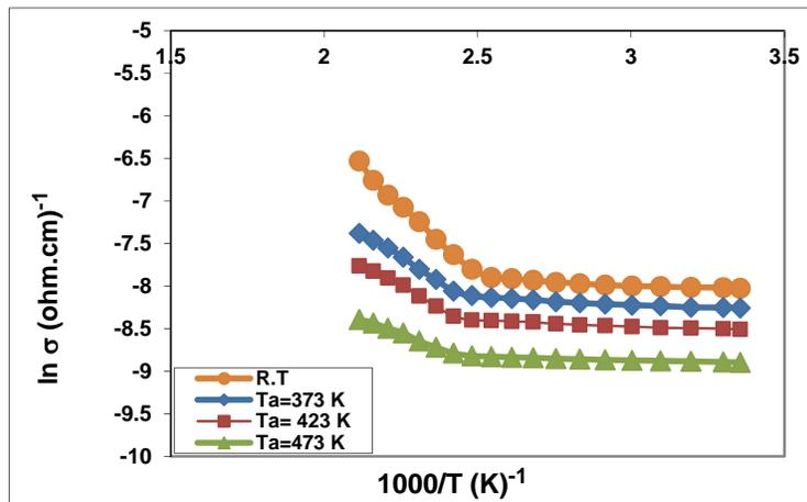
Figure No. (3):  $\ln \sigma$  versus  $10^3/T$  as a function of annealing temperature for (CdTe) films
