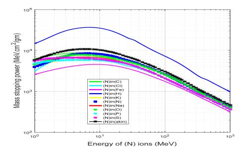
Figure (1): Mass stopping power for nitrogen in elements presented in skin using SRIM program
