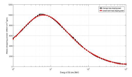
Figure (4): Comparison mass stopping power for N with skin tissue calculated by P.W and average of four methods
