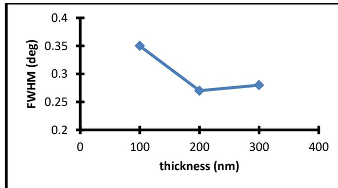
**Figure (2): FWHM vs thickness on ZnO thin films.**
