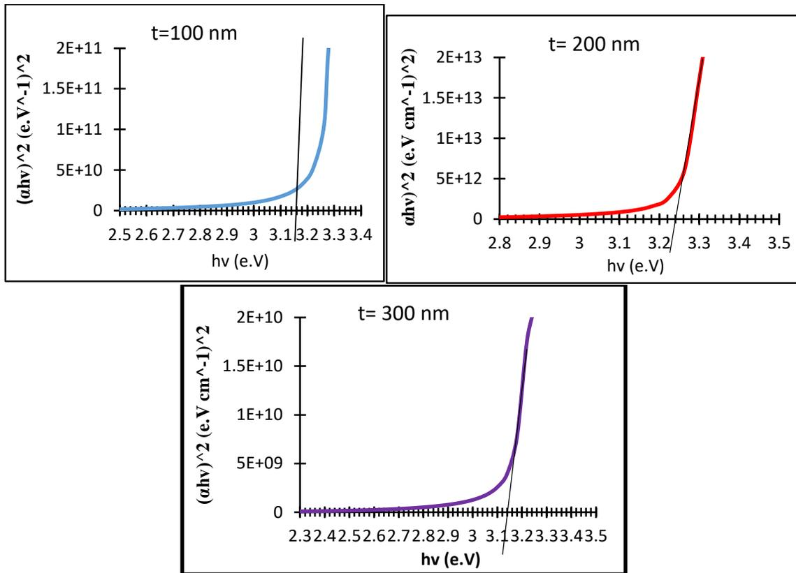
**Figure (5): A plot of  $(\alpha h\nu)^2$  as function of photon energy for ZnO films with different thicknesses.**
