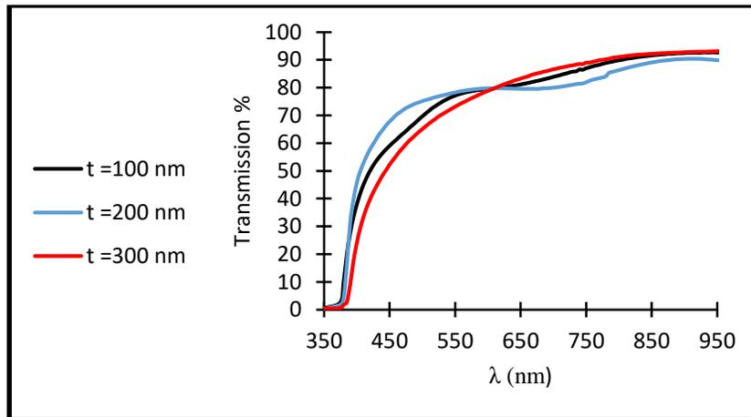
Figure (4): Transmission of ZnO thin films with different thicknesses.
