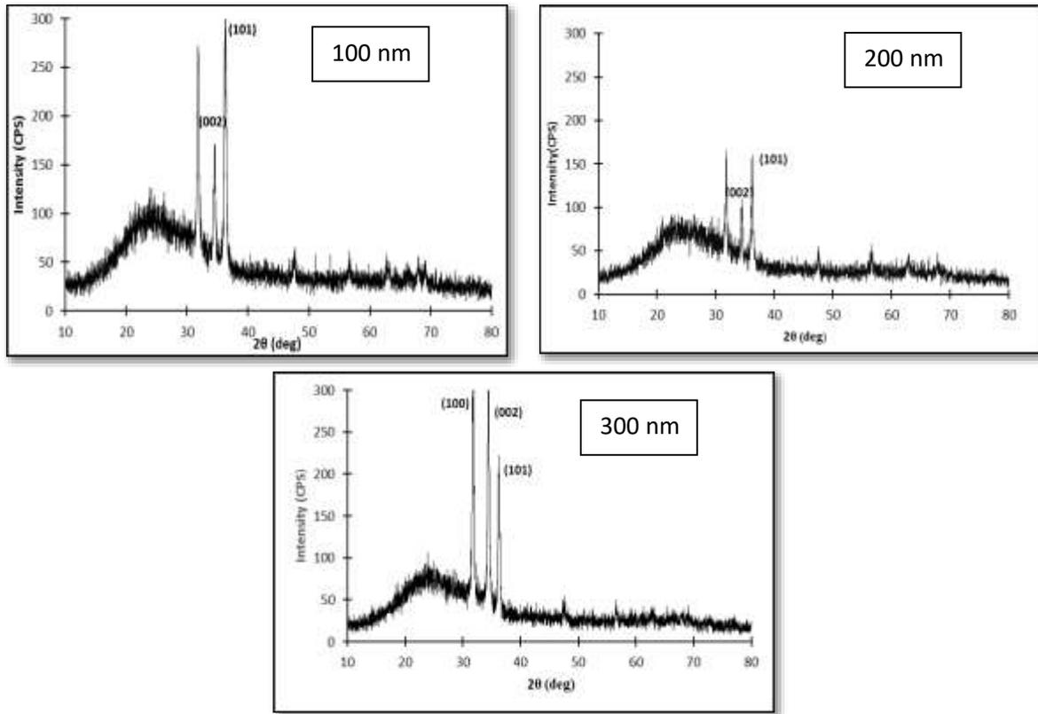
**Figure (1): XRD patterns of ZnO thin films at a different thicknesses (a) 100 (b) 200 and (c) 300 nm.**
