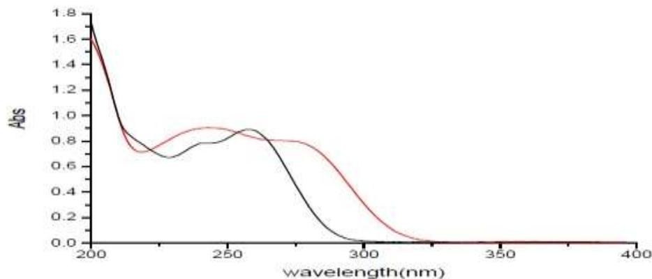
Figure (2): zero order spectra of 4-Aminoantipyrene 30 mg/l (red) and acidic product 30 mg/l (black).
