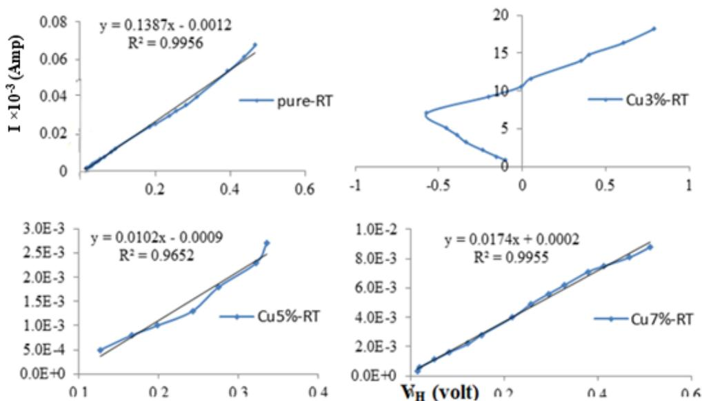
**Figure 3.** Hall voltage relationship and the current passing through pure and doping Cu thin films prepared at room temperature
