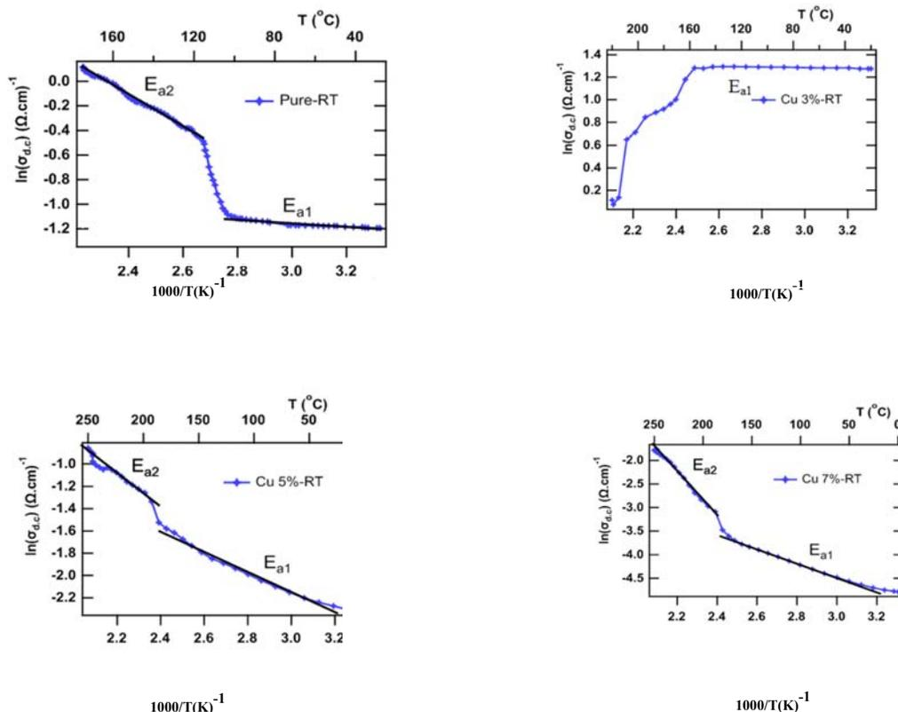
**Figure 2.**  $\ln(\sigma_{dc})$  versus  $10^3/T$  for ZnTe films at different ratio of Cu.
