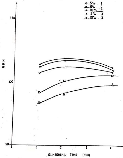
Fig. (3) Variation of hardness with sintering time.
