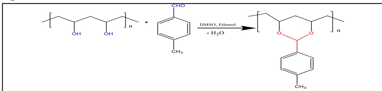
**Figure 1.** Synthesis of polyacetal.
