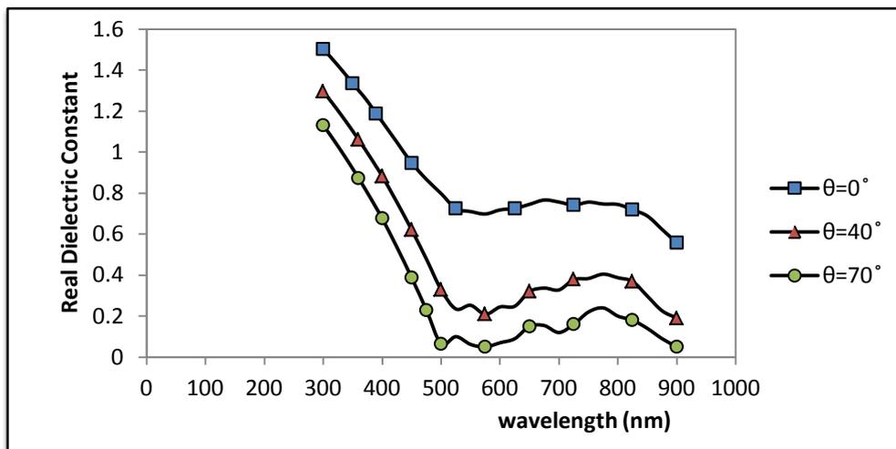
Figure No.(6): Relation between Real Dielectric constant and wavelength with different deposition angles
