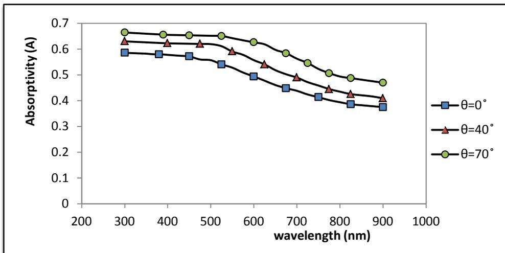
Figure No.(3): Relation between Absorbance and wavelength with different deposition angles
