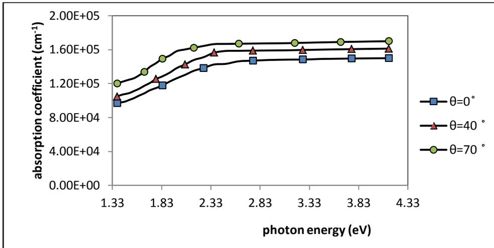
Figure No.(4): Relation between absorption coefficient and photon energy with different deposition angles
