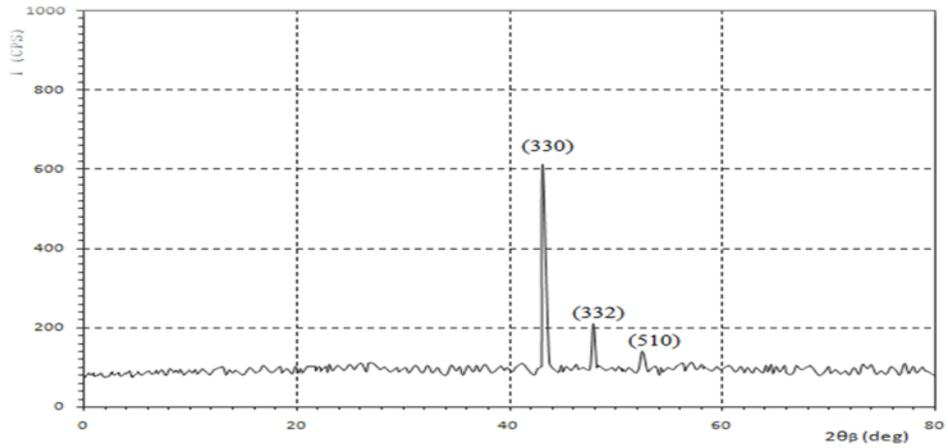
Figure No.(1) : XRD of Mn film deposited at  $\theta=0^\circ$
