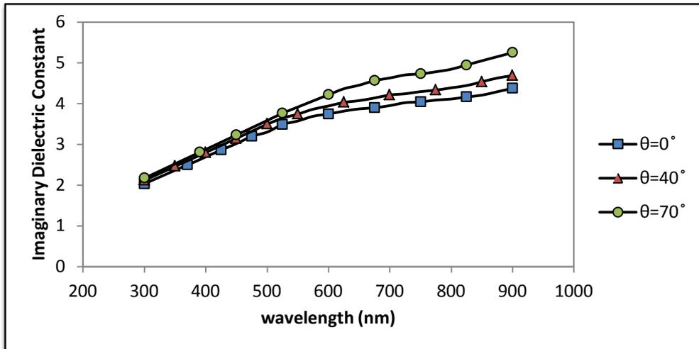
**Figure No.(7): Relation between Imaginary Dielectric constant and wavelength with different deposition angles**
