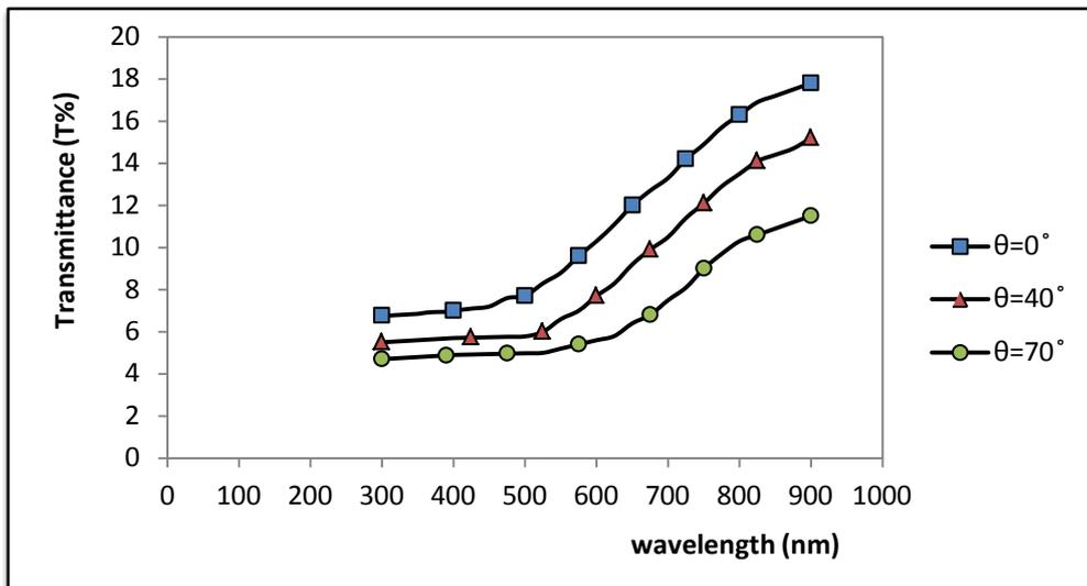
Figure No.(2) Relation between transmittance and wavelength with different deposition angles
