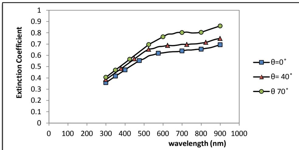
Figure No.(5) Relation between Extinction Coefficient and wavelength with Different deposition angles
