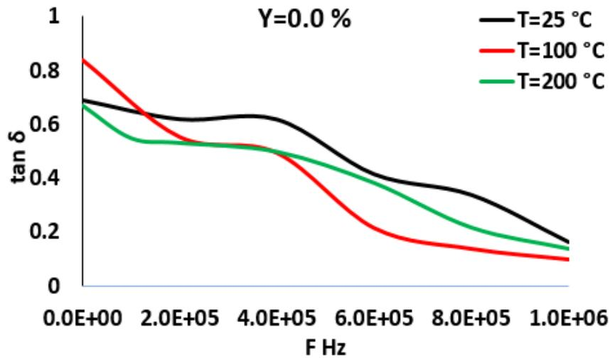
Figure 10. Tangent as a function of frequency for the  $\text{PbSr}_2\text{Ca}_2\text{Cu}_3\text{O}$  compound
