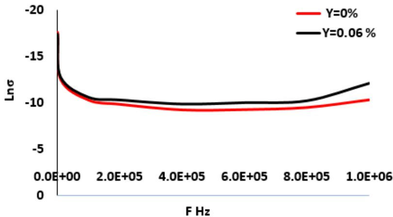
**Figure 5.** Electrical Conductivity as a function of frequency for the  $\text{PbSr}_2\text{Ca}_2\text{Cu}_3\text{O}$  and  $\text{pbSr}_2\text{Ca}_2\text{Cu}_{2.4}\text{Zn}_{0.6}\text{O}$  compounds
