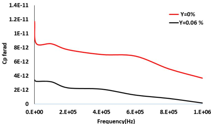
**Figure 2.** Capacitance of the  $\text{PbSr}_2\text{Ca}_2\text{Cu}_3\text{O}$  and  $\text{PbSr}_2\text{Ca}_2\text{Cu}_{2.4}\text{Zn}_{0.6}\text{O}$  compounds.
