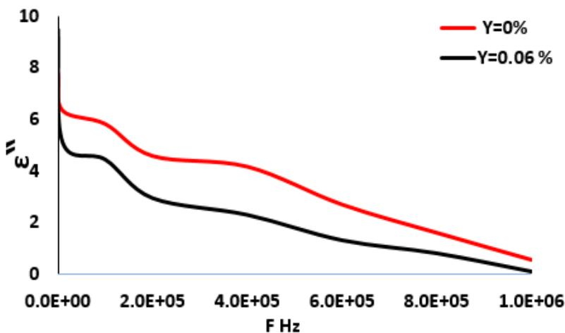
**Figure 4.** Variations in the imaginary dielectric constant as a function of frequency for the  $\text{PbSr}_2\text{Ca}_2\text{Cu}_3\text{O}$  and  $\text{pbSr}_2\text{Ca}_2\text{Cu}_{2.4}\text{Zn}_{0.6}\text{O}$  compounds
