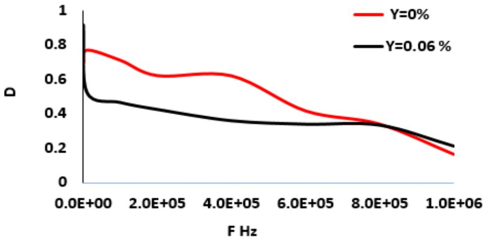
**Figure 3.** Variations in the dielectric constant as a function of frequency for the  $\text{PbSr}_2\text{Ca}_2\text{Cu}_3\text{O}$  and  $\text{pbSr}_2\text{Ca}_2\text{Cu}_{2.4}\text{Zn}_{0.6}\text{O}$  compounds
