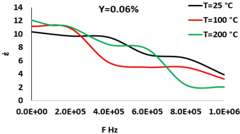
**Figure 7.** Real Dielectric Constant as a function of frequency for the  $\text{PbSr}_2\text{Ca}_2\text{Cu}_{2.4}\text{Zn}_{0.6}\text{O}$  compound as a function of temperature
