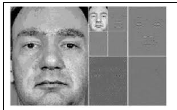
Figure (3) : An Example of Two-Level Wavelet Decomposition of a Face Image.
