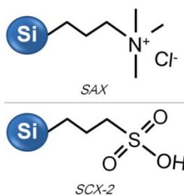
**Figure (1) :Structure of the sorbents (SAX and SCX-2) used for ionic compounds characteristics**
