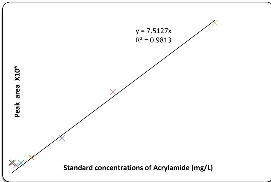
**Figure (3) :** Calibration curve of acrylamide in water
