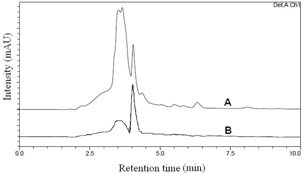
**Figure (2):** Comparison of two overlaid chromatograms showing the enhancement obtained after the use of SPE clean-up for Potato Chips samples; (A) before SPE clean-up (B) after SPE clean-up step.
