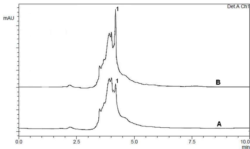
**Figure(4) :**Comparison of two overlaid graphs showing the resulting hplc chromatograms for a sample: (A) neat; (B) spiked with acrylamide. Spiking is accomplished for samples before SPE clean-up. Peak 1 is for acrylamide.
