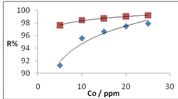
**Fig. (3):** Effect of initial dye concentration on equilibrium adsorption of BG on to (I) bentonite (II) Fe-BNC
