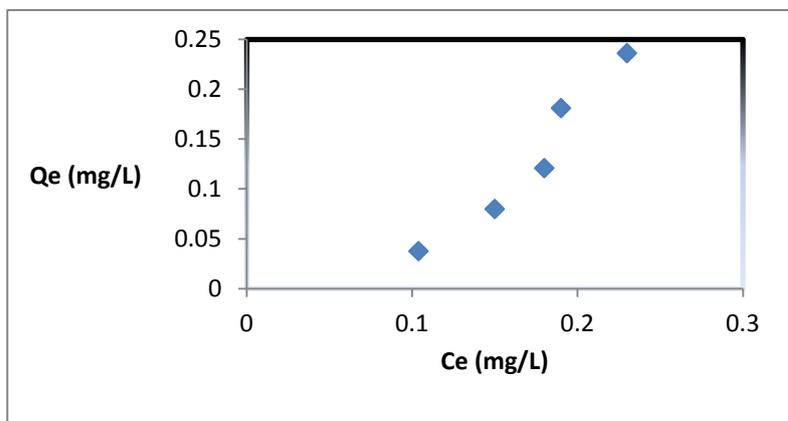
**Fig. (9):** Adsorption isotherm of BG on Fe-BNC at 298 K
