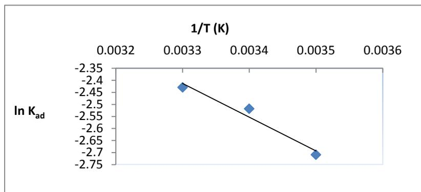
**Fig. (6):** Arrhenius equation of adsorption of BG on Fe-BNC
