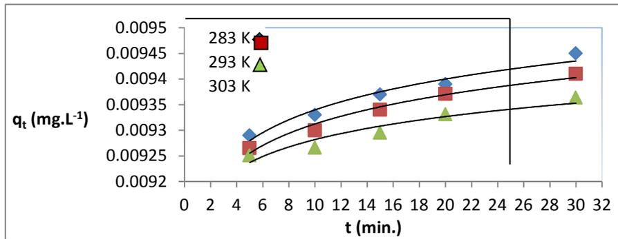
**Fig. (4):** Kinetics of BG uptake by Fe-BNC at several initial temperatures
