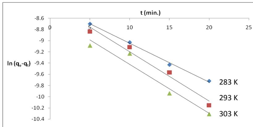
**Fig. (5):** Lagergrens plot for kinetic modeling of the adsorption process of BG on Fe-BNC clay at different temperatures
