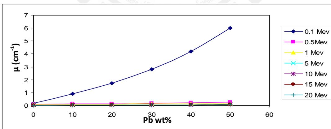
Fig .(2): Total linear attenuation coefficient ( $\mu$ ) as a function of concentration of (Al, Fe and Pb) at different energies
