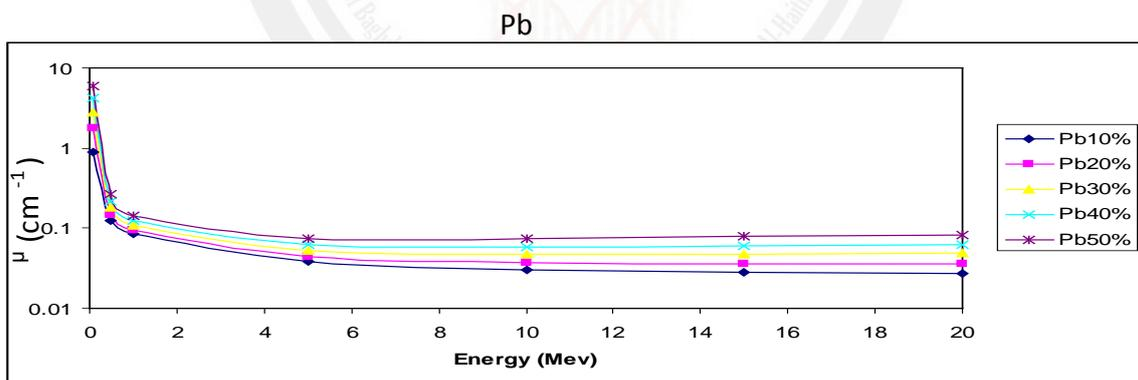
Fig.(1): Total linear attenuation coefficient ( $\mu$ ) as a function of energy (E) at different concentrations of (Al, Fe and Pb)
