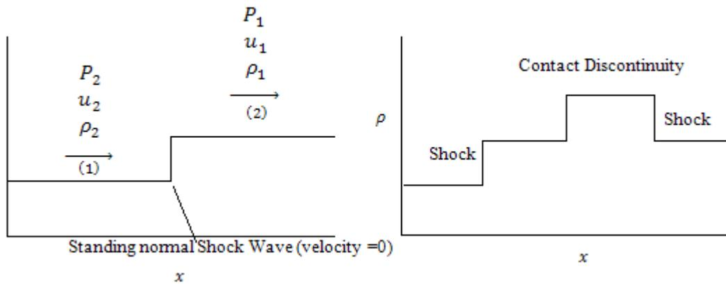
Fig( 2): Collision of two flows
