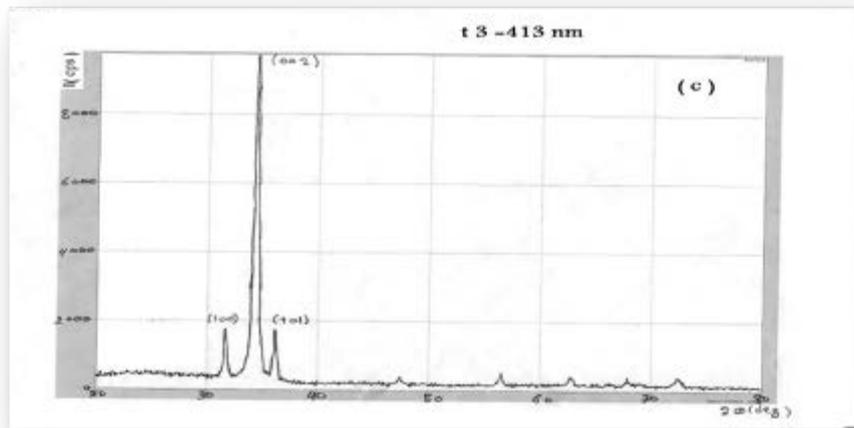
Fig. (1): XRD spectrum of ZnO films with different thickness (A) 222nm, (B) 317nm and (C) 413nm
