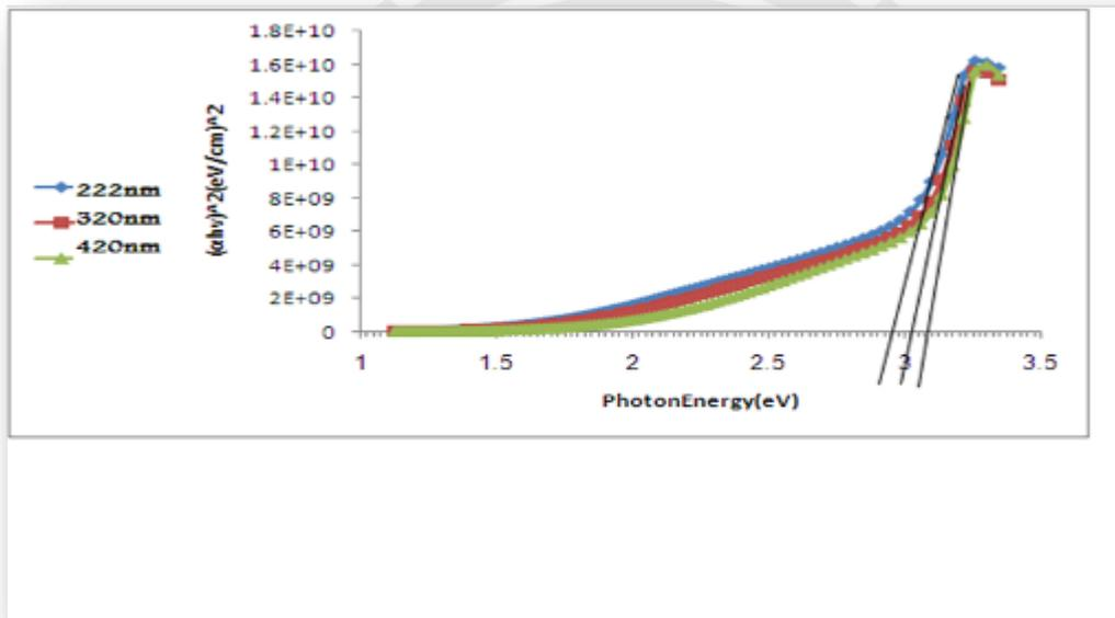
Fig. (4): A plot of  $(\alpha h\nu)^2$  as function of photon energy for ZnO films with different thicknesses
