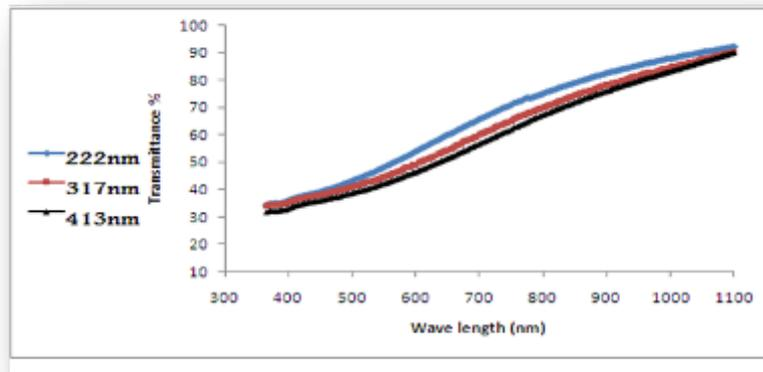
Fig.(3): Transmission as function of wavelength for ZnO films with different thicknesses
