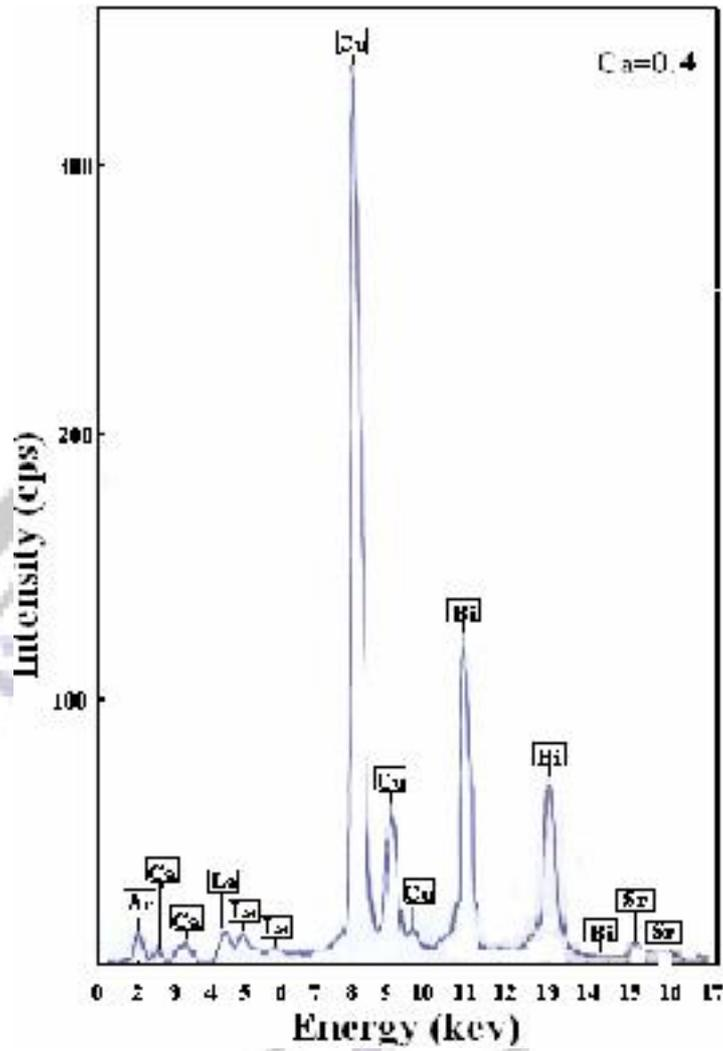
Fig.(3): XRF Patterns for the sample  $\text{Bi}_2\text{Sr}_2\text{La}_{2-x}\text{Ca}_x\text{Cu}_3\text{O}_{10+\delta}$  for  $x=0.4$
