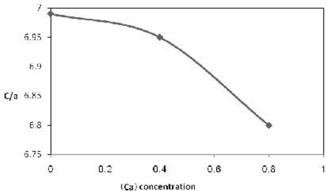
Fig.(6): C/a as function of different Ca for  $\text{Bi}_2\text{Sr}_2\text{La}_{2-x}\text{Ca}_x\text{Cu}_3\text{O}_{10+\delta}$
