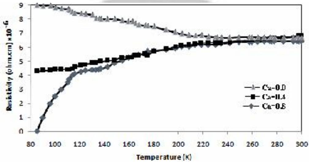
Fig. (1): The resistivity dependence on Temperature for  $\text{Bi}_2\text{Sr}_2\text{La}_{2-x}\text{Ca}_x\text{Cu}_3\text{O}_{10+\delta}$  at indicated values of (Ca) at  $x=0.00, 0.4$  and  $0.8$
