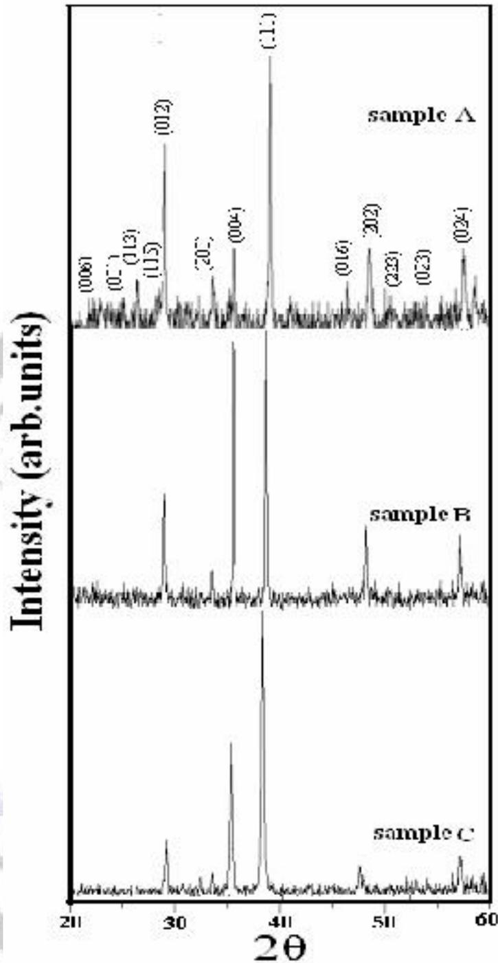
Fig.(5): XRD Patterns for the sample  $\text{Bi}_2\text{Sr}_2\text{La}_{2-x}\text{Ca}_x\text{Cu}_3\text{O}_{10+\delta}$  for A ( $x=0.0$ ),
