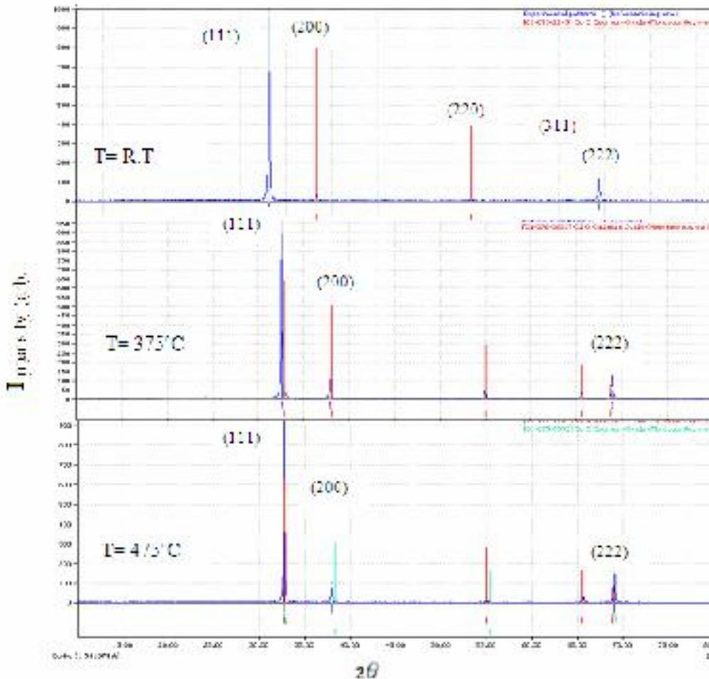
Fig.( 1): X-Ray diffraction of the CdO thin films. before and after annealing temperatures
