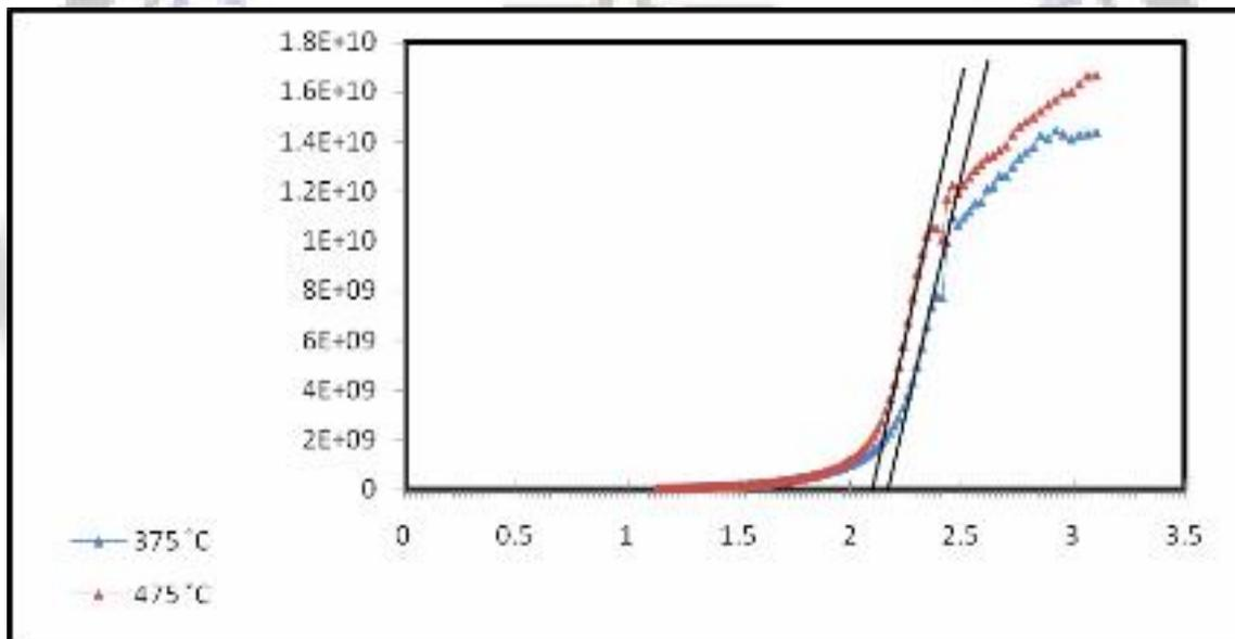
Fig.(3): The band gap is for direct transition of the CdO films at annealing temperatures: (375and 475) °C, and thickness: (450) nm, as a function of photon energy
