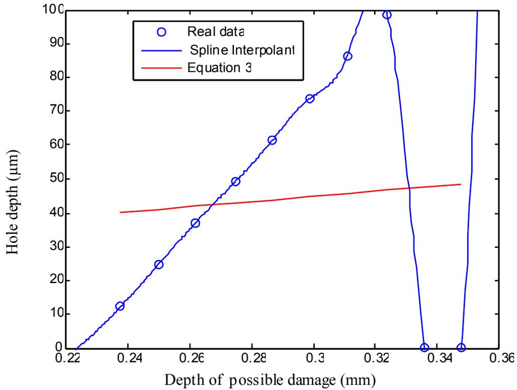
**Fig.(3): Scatter plot and fitted equation for depth of possible damage and hole depth(Copper).**
