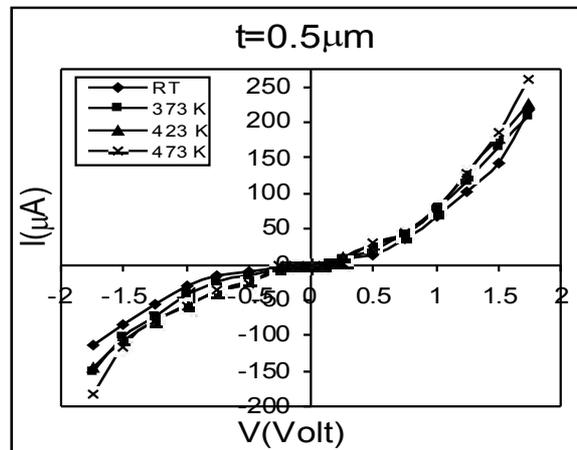
**Fig. (2): I-V characteristics in the dark for a-Ge:Sb/c-Si heterojunction at forward and reverse bias voltage at different annealing temperatures**
