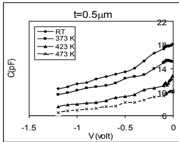
Fig. (3): The variation of capacitance versus reverse bias voltage for a-Ge:Sb/c-Si heterojunction for different annealing temperatures
