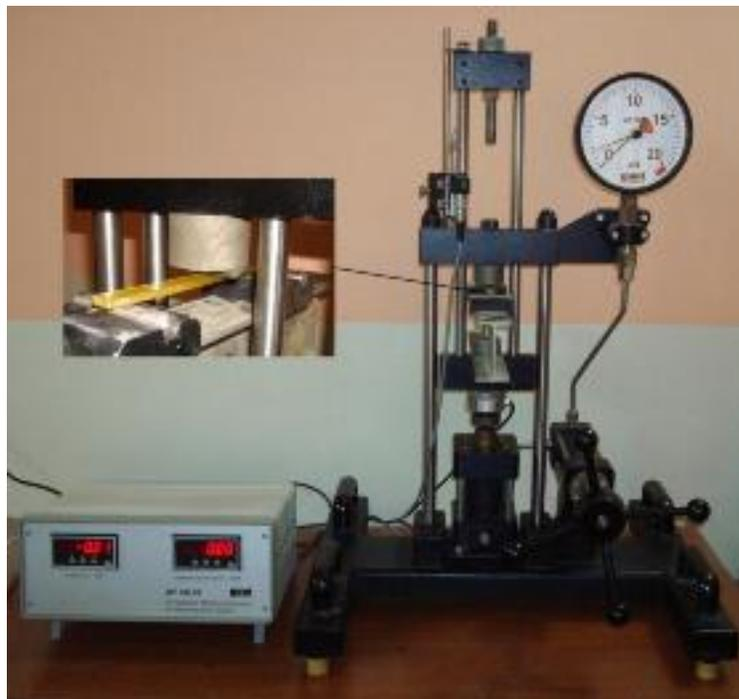
**Fig.(2): Flexural test-rig with an exploded view of the matrix material test specimen under three-point bending load**
