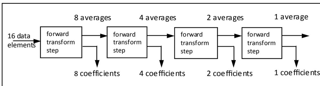
**Fig. (3): 4 steps of a 16 element wavelet transform.**
