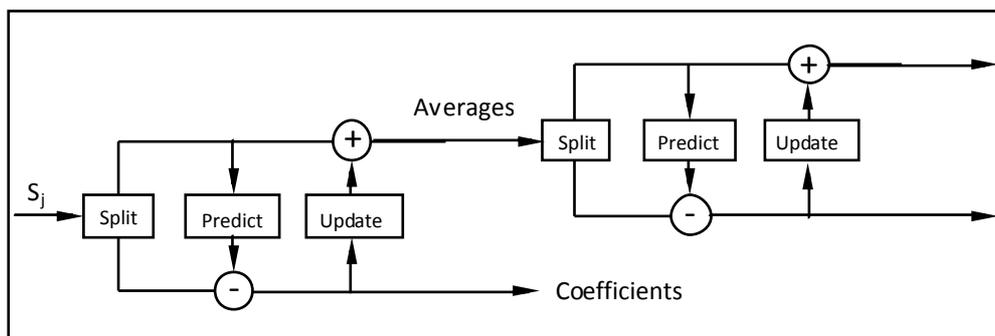
**Fig. (2): Two steps in the wavelet lifting scheme Haar forward transform.**
