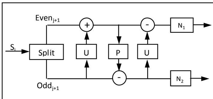
Fig. (5): Forward transform step of the lifting scheme version of the Daubechies D4
