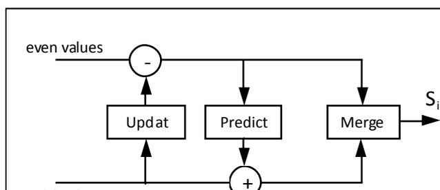
Fig. (4): Lifting scheme inverse transform.
