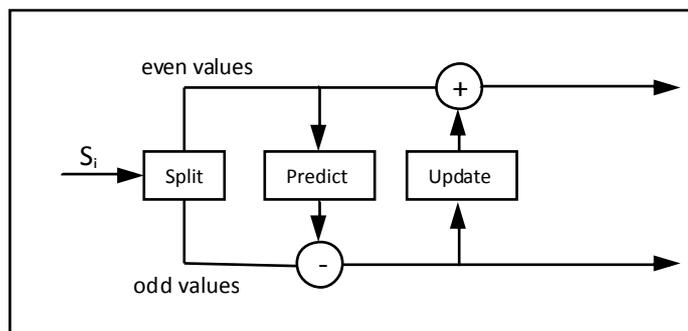
**Fig. (1): Lifting scheme forward wavelet transform.**
