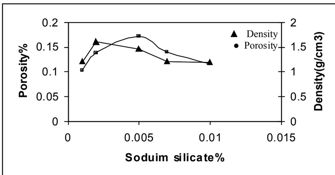
Fig.(4) The apparent density and porosity with concentration of sodium silicate for samples firing at 1250 °C
