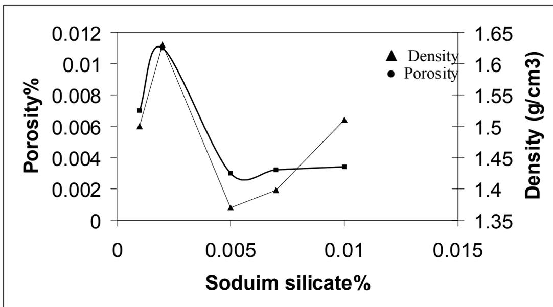
Fig.(3) The apparent density and porosity with concentration of sodium silicate for samples firing at 1350 °C
