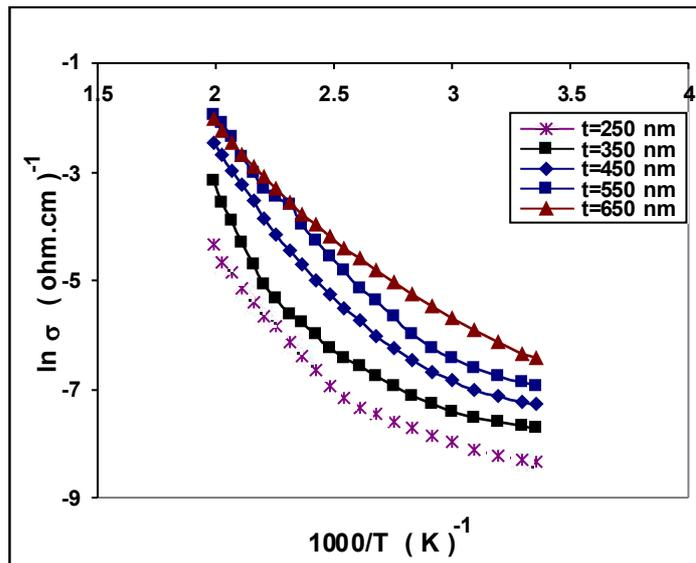
Fig.(1): Electrical conductivity behaviour as a function of temperature for a-InAs thin films as-deposited at different thicknesses.
