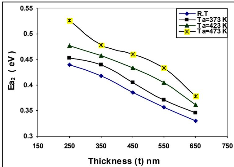
Fig.(3):Activation energies versus thickness of a-InAs thin films at different annealing temperatures
