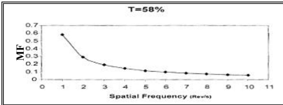
Fig. (6) The MF with the spatial frequency at transmittance 58%
