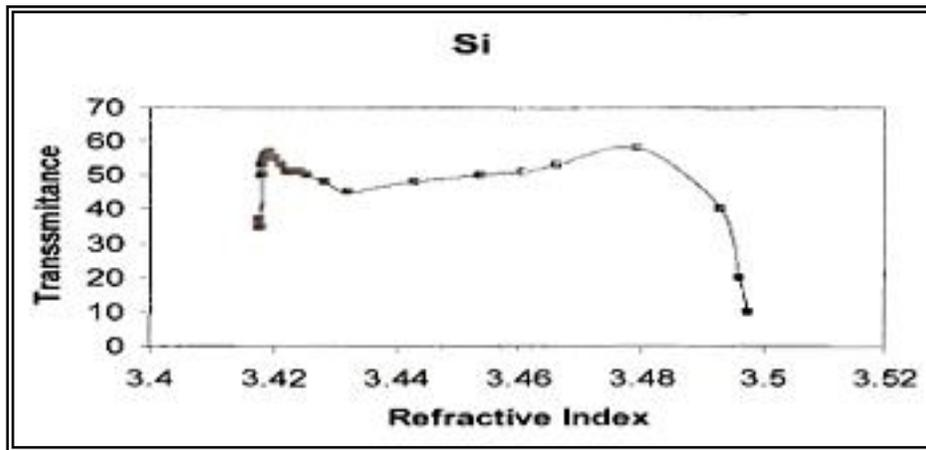
Fig. (2) The transmittance with refractive index for silicon
